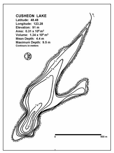
Figure 2. Cusheon Lake Bathymetric Map (from Spafard, S.A, et al., 2002).
