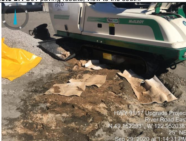
Photo 29. Oil spill from the pipe fuser machine at River Road west.
