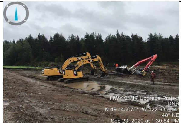
Photo 10. Rescue mission of excavator sunk in the DNR.
