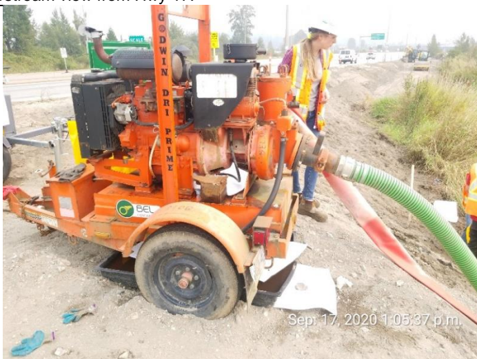
Photo 17. A fitting on a water pump was leaking oil into the secondary containment which had filled with water and overflowed.
