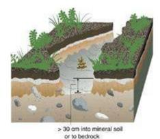
Deep gouges are excavations into mineral soil that are deeper than 30 cm or to bedrock at the survey point.
