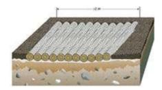
*Corduroyed trails* are constructed using logs and woody debris placed side by side to form a surface greater than 2 m in length and capable of supporting equipment traffic.
