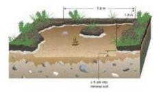
*Wide gouges* are excavations into mineral soil that are a) deeper than 5 cm at the survey point and b) deeper than 5 cm or to bedrock, on at least 80% of an area 1.8 x 1.8 m.
