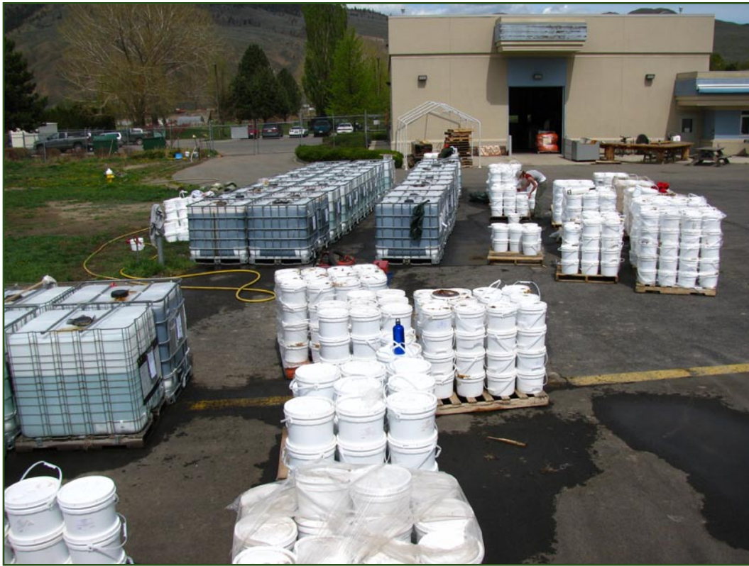
Water and molasses mixture being prepared at the Kamloops Fire Centre. The large containers are the 1,000 litre bulks used to hold the spray mixture, and the white buckets are some of the 14,000 litres of molasses that was hand-mixed into the water.
