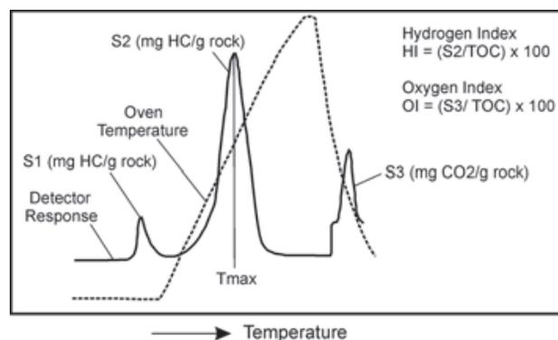
Figure 9. Schematic pyrogram illustrating the liberation of hydrocarbon during heating of the rock sample. Determined parameters include S<sub>1</sub>, S<sub>2</sub>, S<sub>3</sub>, T<sub>max</sub>, and the hydrogen and oxygen indices.
