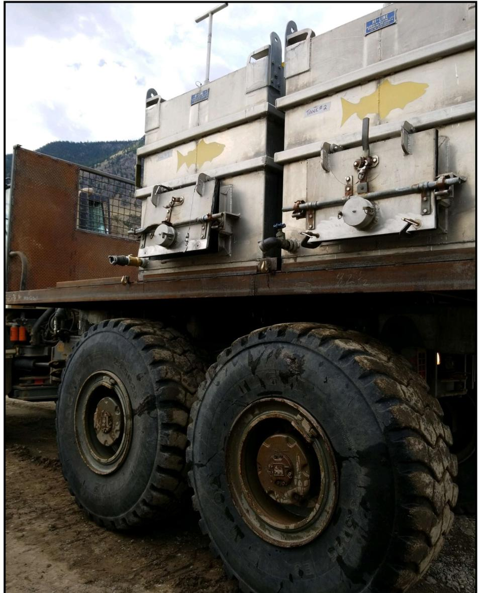
**PICTURED:** When needed, salmon will be transported in specially designed 2,700-litre tanks fitted to flat-bed trucks
