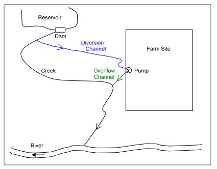
Figure 3.3 Conveyance Loss Example
