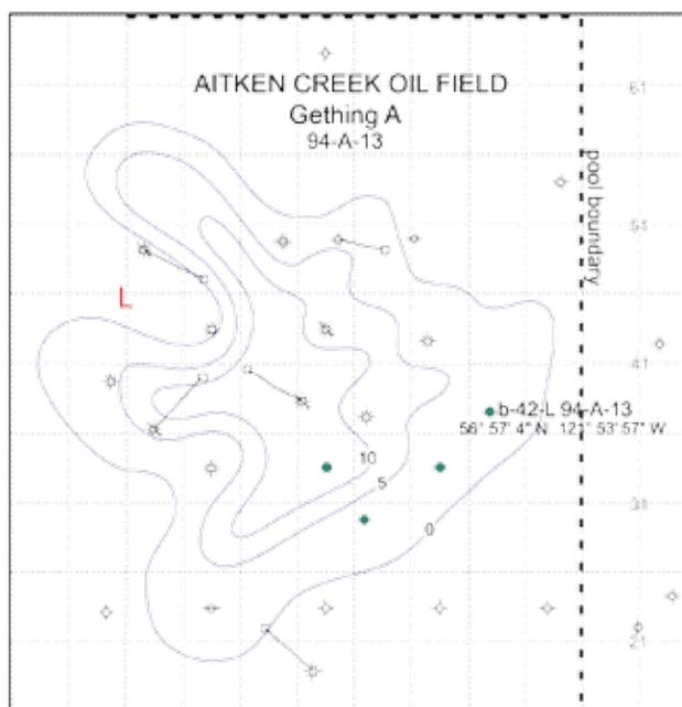
Figure 1: Example of a map provided for each pool profiled in the upcoming open file release. Contour interval is 5 m net Gething A oil pay, and the discovery well is b-42-L-94-A-13. The entire updip portion of the pool (northwest) is undrained by oil wells and gas is being injected into the updip side of the pool (contours are from the British Columbia Oil and Gas Commission).
