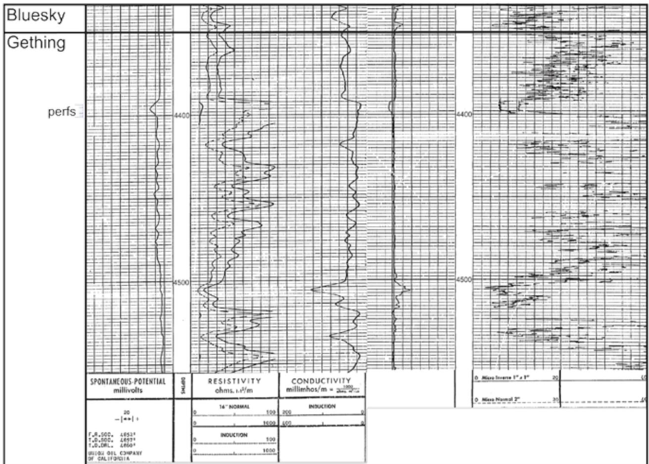
Figure 2: Example of representative wireline logs provided for each pool profiled in the upcoming open file release: elog and microlog for discovery well b-42-L-94-A-13. The microlog indicates good permeability across the perfed interval (4392'–4400').
