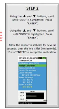
NOTE: Use DO% (%Saturation) when calibrating the Dissolved Oxygen, but use mg/L when recording Dissolved Oxygen values on the field sheets.
