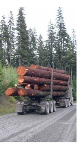
The amount of payload influences the stability of truck & trailer combinations. A dynamic stability analysis may be necessary to determine if a truck is safe to drive under the intended road and loading conditions.
