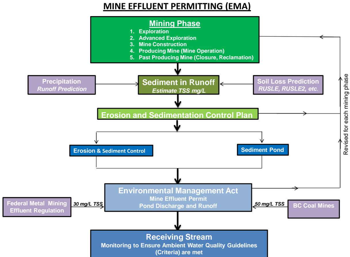
Figure 1 provides the methodology that the Qualified Professional should apply when developing and applying an Erosion and Sediment Control Plan. Note that each phase of mine development beyond exploration requires an *Environmental Management Act* permit.
