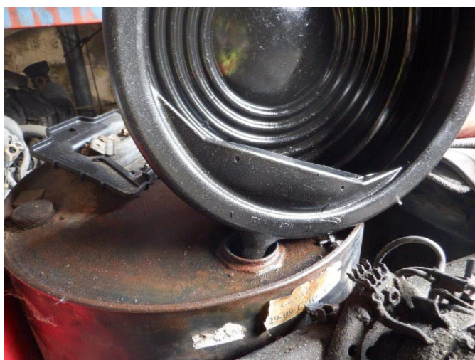
Photo 2 – Oil pan stored in the opening of an unlabelled hazardous waste storage drum
