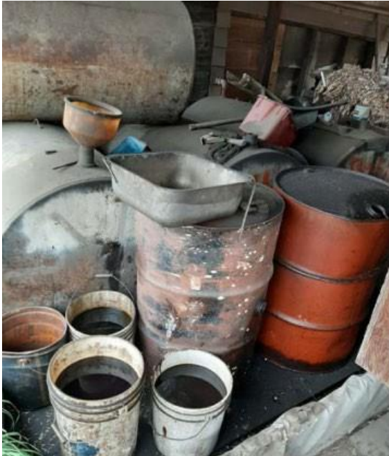
Photo 3 –Hazardous waste stored in open pails and all of the containers are unlabelled.
