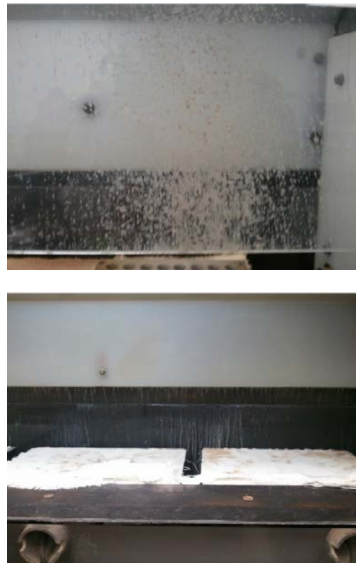
Figure 2. (Top) Build-up of unknown material on fume hood sash. (Bottom) Build-up of material on wash-down screen. Build-ups of material such as these should be avoided by implementing a regular cleaning schedule.
