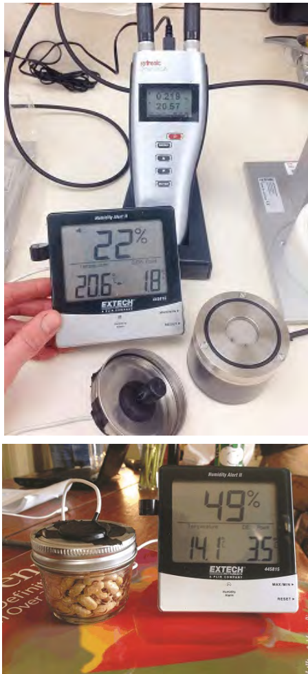
Figure 1. Comparing my Extech hygrometer to the Rotronic HydroPalm 23-AW at the National Tree Seed Centre, top. Testing a batch of garden Phaseolus for long-term potential. Adjusted eRH% at 20°C is 33.7%, bottom.
