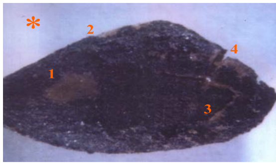
Figure 2. * Highlighted seed; 1) abrasion; 2) chip; 3) crack; 4) seed breakage
