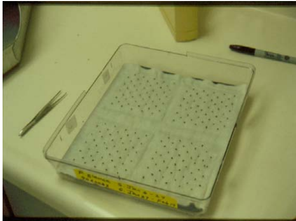
Figure 1. Seed on vacuum seed head (top) and four replicates of 50 seed each on moistened VersaPak™ (bottom).
