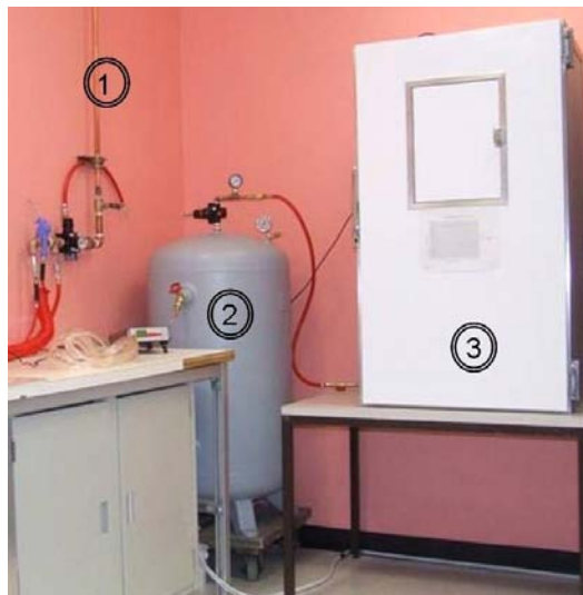
Figure 2. Seed and/or pollen dryer monitored with a_w . 1- air pressure distribution, 2- saturation tank, 3- cabinet for seed or pollen equilibration.
