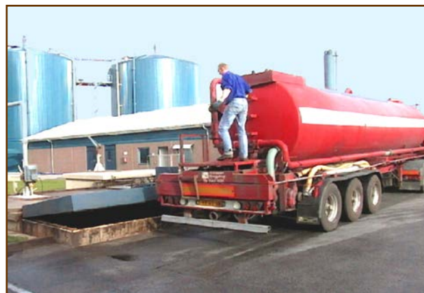
Figure 3 A tanker truck unloading non-agricultural waste into a sealed underground pre-storage tank (for odour control) at a large scale co-digestion biogas plant in Denmark run by a farm cooperative.
