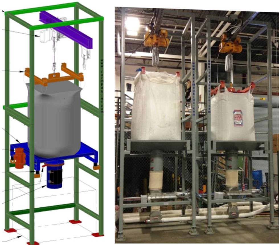
Figure 2: Example of the Bag Handling Component of a Dry Powder System (graphics by FormPac, Inc.)
