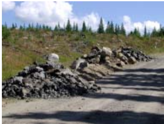
Figure 3. Stockpiled aggregate showing one load of riprap on either end of the crushed rock.
