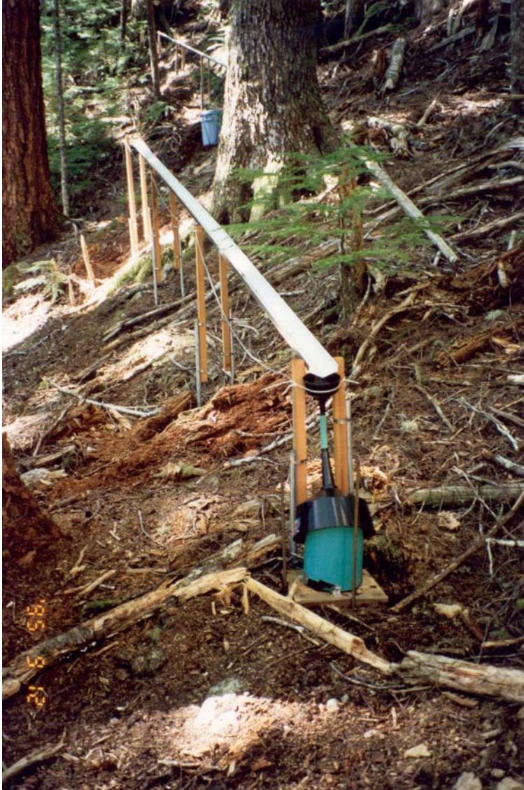
Hydrologic Recovery Studies. Rainfall interception and runoff measurement in old-forest site.
