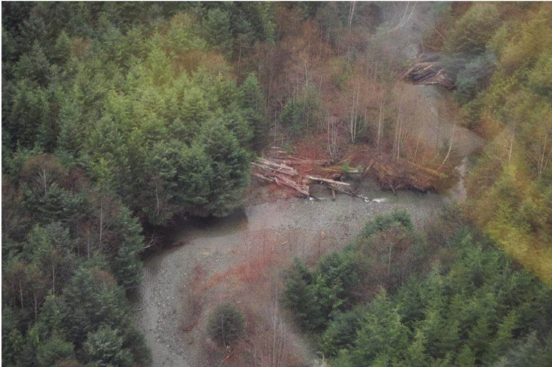
Large logjams and associated sediments deposited by debris torrents in 1984 have moved progressively downstream through the clearcut riparian treatments to the leave-strip zone.
