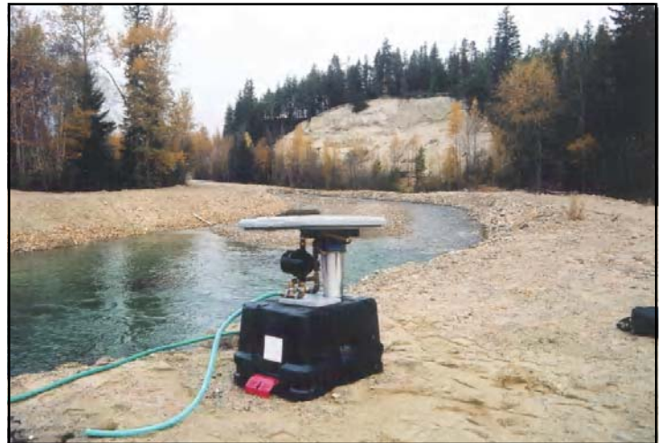
Plate 3. The parasite filtration kit on the bank of Swift Creek beside the water pump house.
