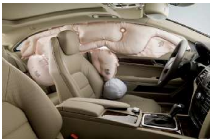
Side head curtains and air bags to protect the thorax are examples of how vehicle technology helps protect the human head and body from blunt crash force.
