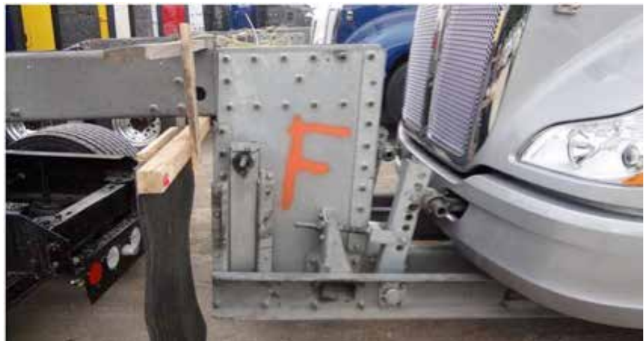
Figure 3: Tow eye connection of the forward extended saddle system
