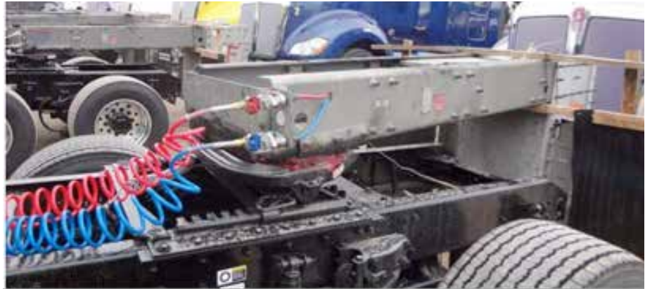
Figure 2: Roll-coupled connection to lead vehicle
