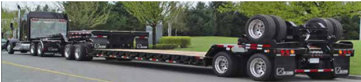
Figure 1: Tractor, Tandem Jeep, Tandem Double Drop Trailer with Flip-up Booster
