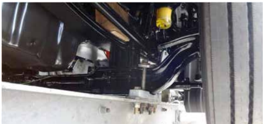
Figure 4: Steer axle clamp connection of the forward extended saddle system
