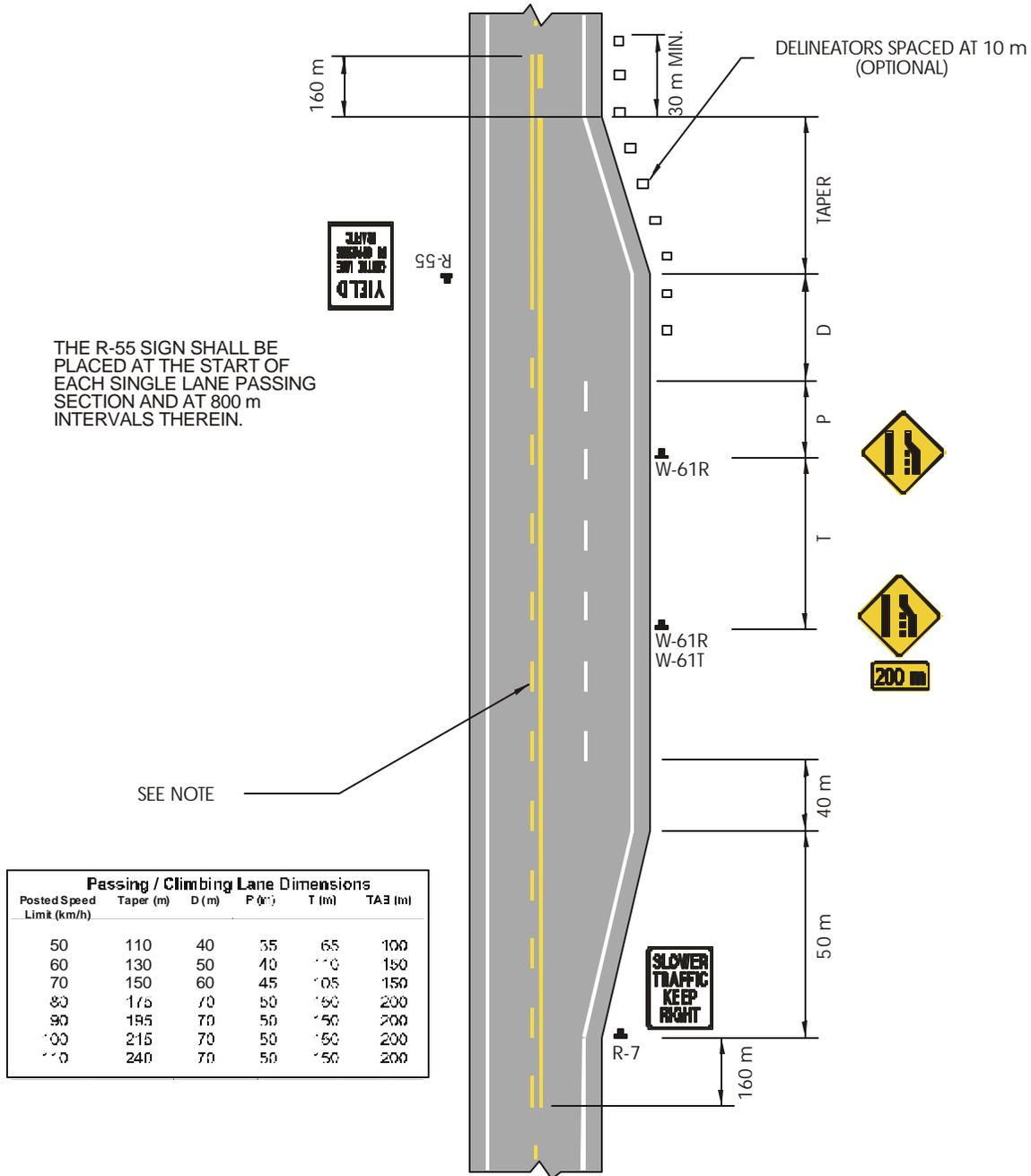
NOTE: CONTINUOUS BARRIER LINES SHALL BE MARKED IN THE SINGLE LANE DIRECTION REGARDLESS OF THE SIGHT DISTANCE UNLESS APPROVED FOR DOWNHILL PASSING BY THE SENIOR TRAFFIC ENGINEER.
