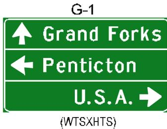
The **G-1, Destination Direction** sign series directs motorists to the next major destination or control city depending upon the geographical setting. These signs shall be erected 100m to 200m in advance of intersections and are typically shoulder mounted. In urban areas, overhead mounting may be desirable if criteria outlined in Sec. 1.9, 'General Provisions', of this manual is satisfied.
