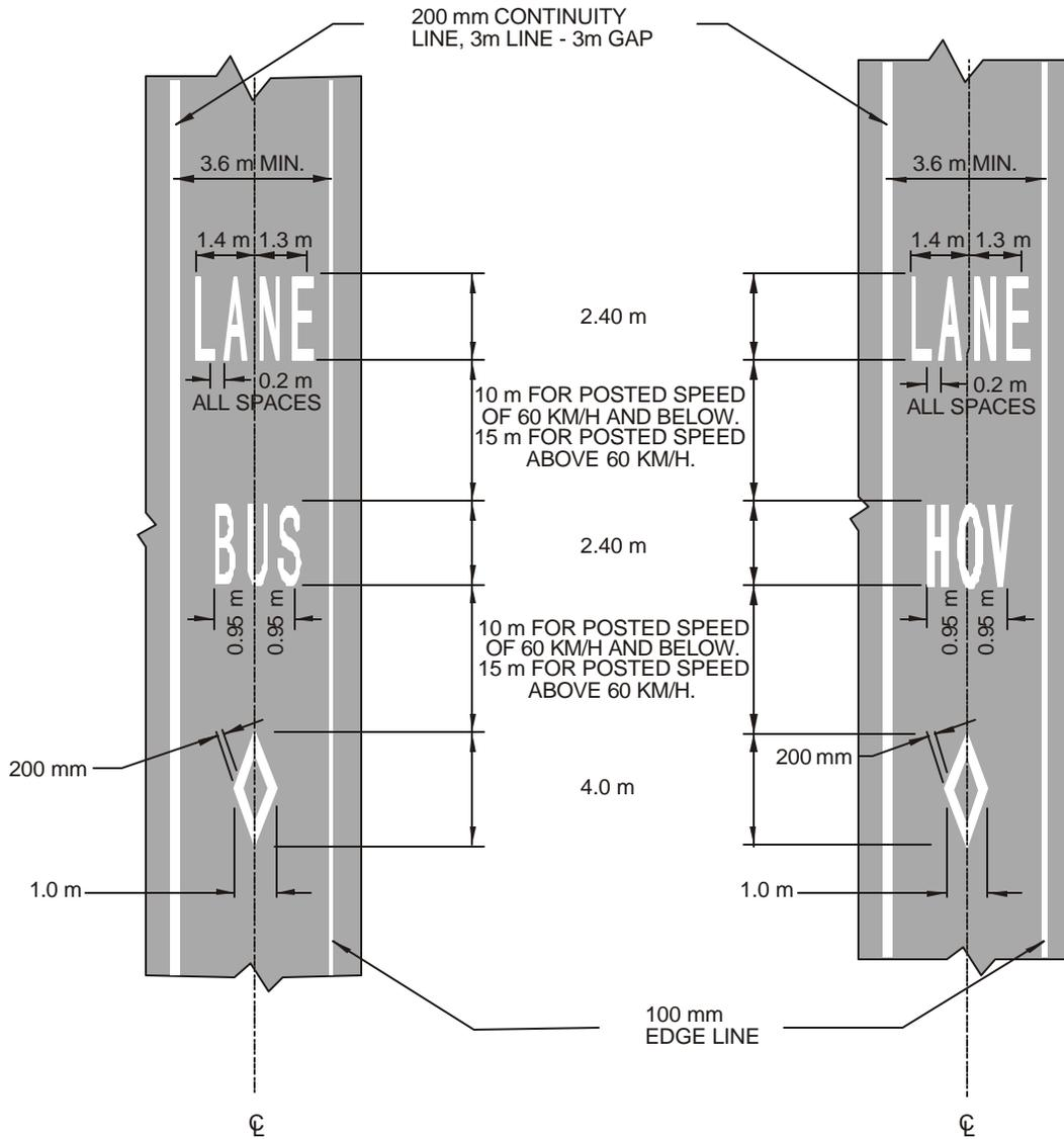
NOTE: BUS AND HOV PAVEMENT MARKING SYMBOLS AND WORDED MESSAGES ARE TO BE REPEATED AT 200 m TO 280 m INTERVALS DEPENDING ON THE OVERALL LENGTH AND CONTINUITY OF THE LANE
