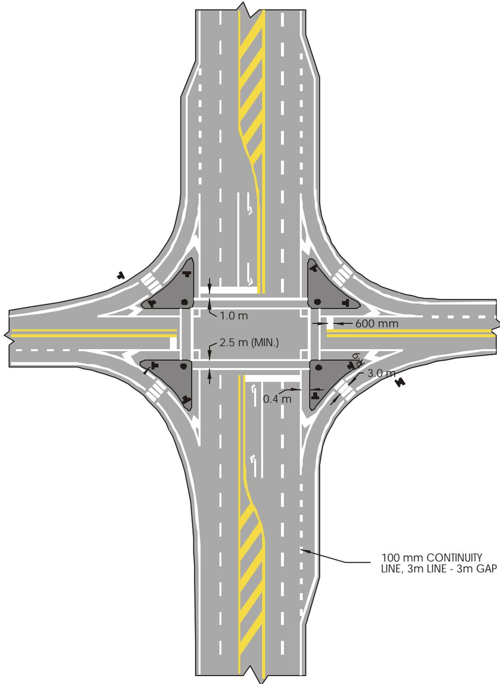
NOTE: WHERE THERE IS NO MARKED CROSSWALK, THE STOP LINE SHALL BE SET BACK FROM THE INTERSECTION TO ALLOW FOR A FUTURE CROSSWALK.
