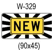
The W-329 NEW tab should be used with the W-12 sign for new signal installations. The NEW tab should remain in place for three months until motorists become familiar with the signal. If the signal has W-116 ADVANCE WARNING flashers, the W-329 and W-12 signs must be removed after the three month education period terminates. The W-329 may also be used with any other standard sign to draw attention to revisions in traffic control.
