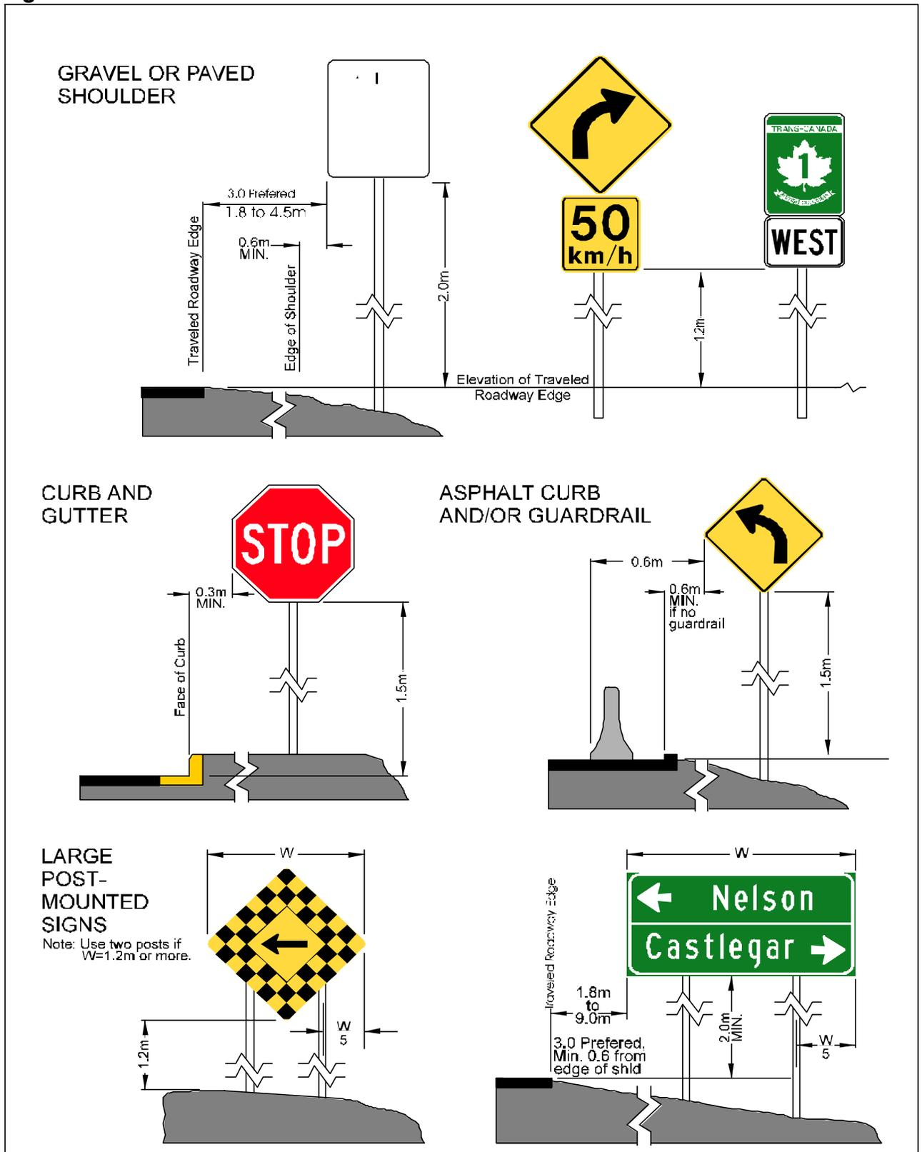
**Fig. 1.2 SIGN HEIGHTS AND LATERAL CLEARANCES**
