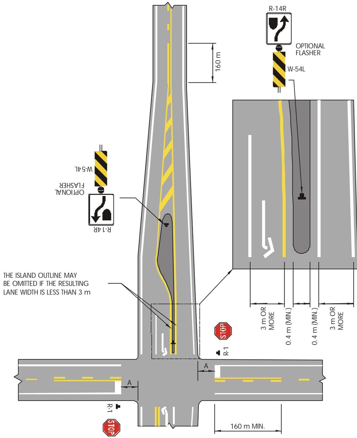
DIMENSION A: WHERE THERE IS NO MARKED CROSSWALK, THE STOP LINE SHALL BE SET BACK FROM THE INTERSECTION TO ALLOW FOR A FUTURE CROSSWALK.
