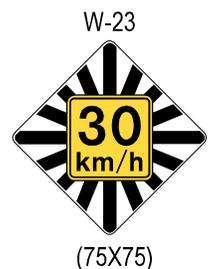
The W-23 signs will display an ADVISORY SPEED tab (W-22) attached at the centre, with the W-23 sign mounted in a diamond shaped orientation. In special circumstances where it is necessary to erect a diamond sign in place of the W-22 tab, the appropriate W-23 sign shall be mounted as a square to allow for a more effective viewing of the W-23 sign's characteristics.
