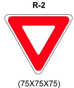
The R-2 sign should be oriented so that motorists on the mainline cannot see the sign face. If this is not practical, the R-2 should be shielded from the mainline motorists by using a visor.
