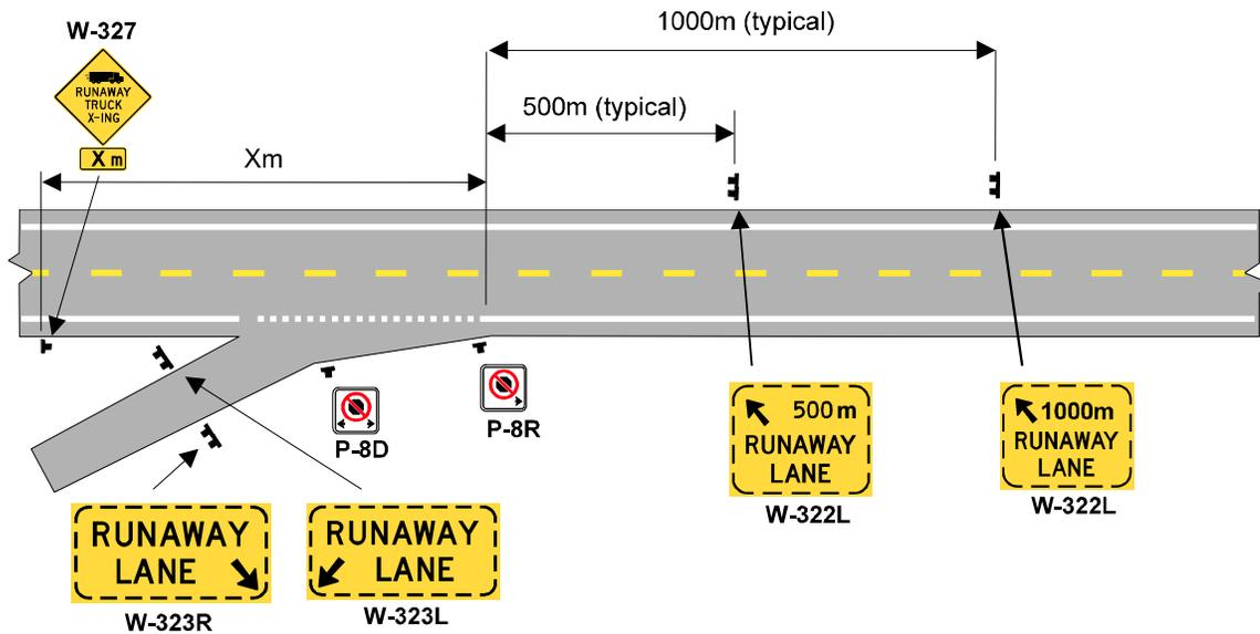
Figure 3.3 Conventional Highway Brake Check
