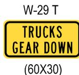
The W-29 sign is also required for hill of any length with a grade of 6% or more, combined with horizontal curves of more than 4 degrees.
