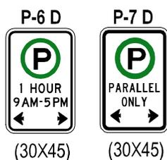
P-6 D/L/R PARKING <TIME LIMITED> signs may be used to permit limited time parking during specified times of day.
