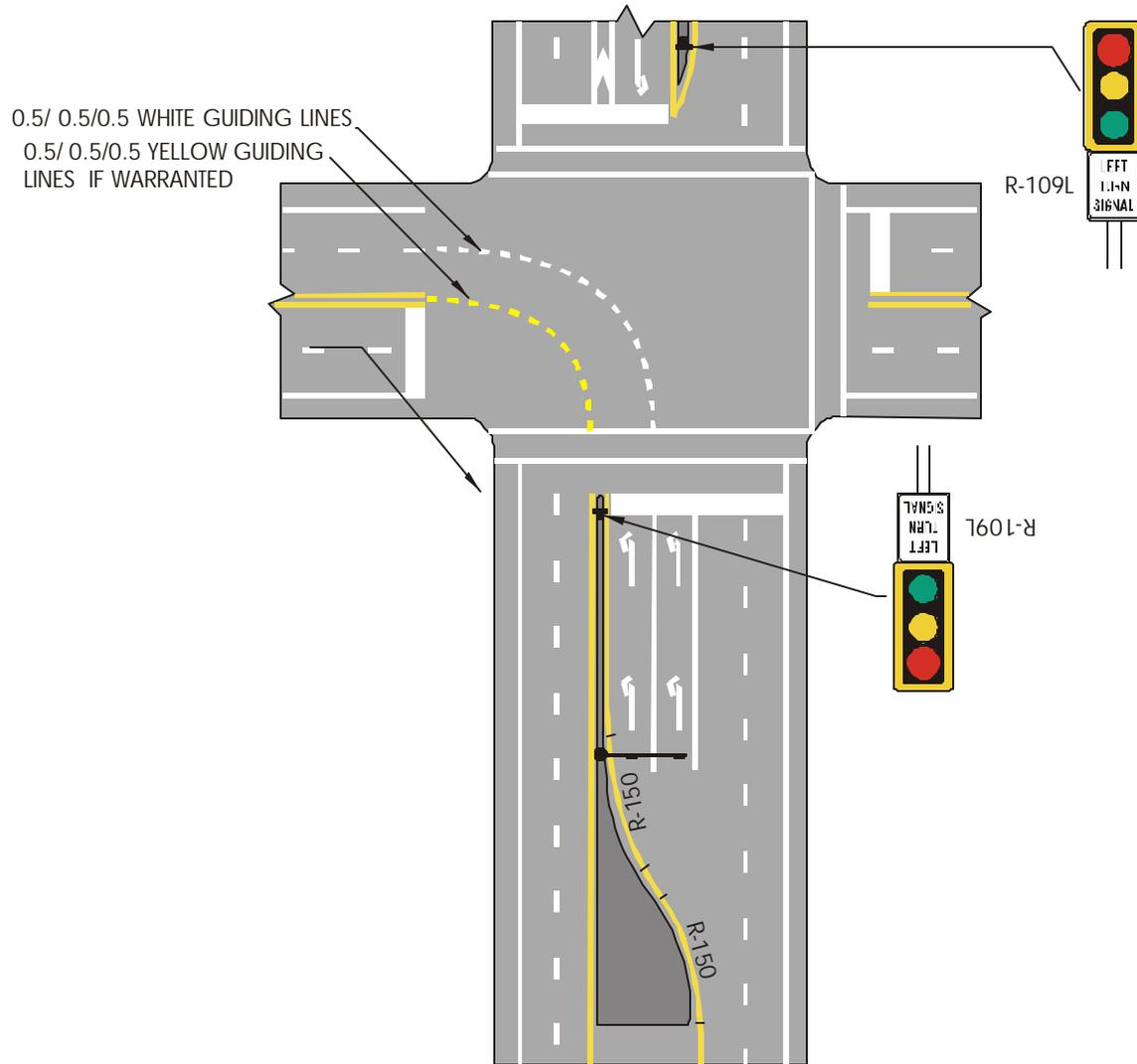
NOTE: GUIDING LINES MAY BE USED FOR SINGLE LEFT TURN LANES IF THE VERTICAL ALIGNMENT AT AN INTERSECTION SECLUDES THE LONGITUDINAL MARKINGS ON THE FAR SIDE OF THE INTERSECTION.
