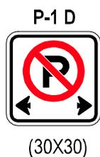
Parking control signs are used to notify the motorist of parking restrictions as specified on the sign. The sign should be erected where the restriction is in effect and be oriented at 30 to 45 degrees from the curb line or road edge so it is visible to the motorist. Signs without arrows should be placed at 90 degrees to the roadway.
