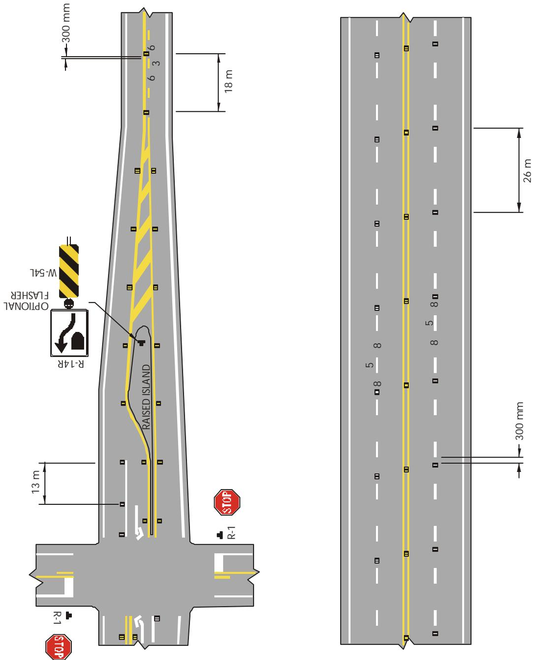
Note: Where the systematic spacing of RPMs is interrupted by a cross street, railway etc., an RPM may be moved in either direction for a distance not exceeding  $\frac{1}{4}$  of the normal spacing. If the RPM still obstructs, it should be left out and the normal spacing continued as though as RPMs were in place.
