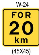
The W-24 ADVISORY DISTANCE tab informs motorists that the condition that the warning sign specifies, exists for a distance of 2 km or more length. The distances shown on the tab should be shown in multiples of 1 km.
