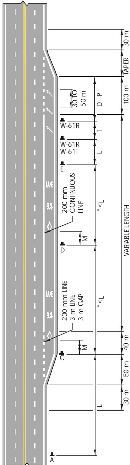
NOTE: SEE Figure 7.37 FOR TAPER, D, P, AND T DIMENSIONS
