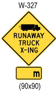
The W-327 RUNAWAY TRUCK CROSSING sign warns of the possibility of runaway trucks crossing the roadway in order to utilize a runaway lane facility located on the left hand side of the down-grade traffic.
