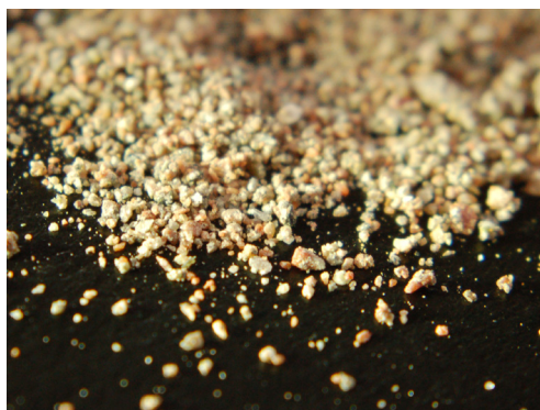
Photo of Mount Polley Mine's tailings. Tailings are particles of ground rock that are left behind after the valuable minerals are extracted. They range in size from sands to fine, clay-sized particles. The geochemical testing program evaluated whether or not they could leach metals or would stay inert.
